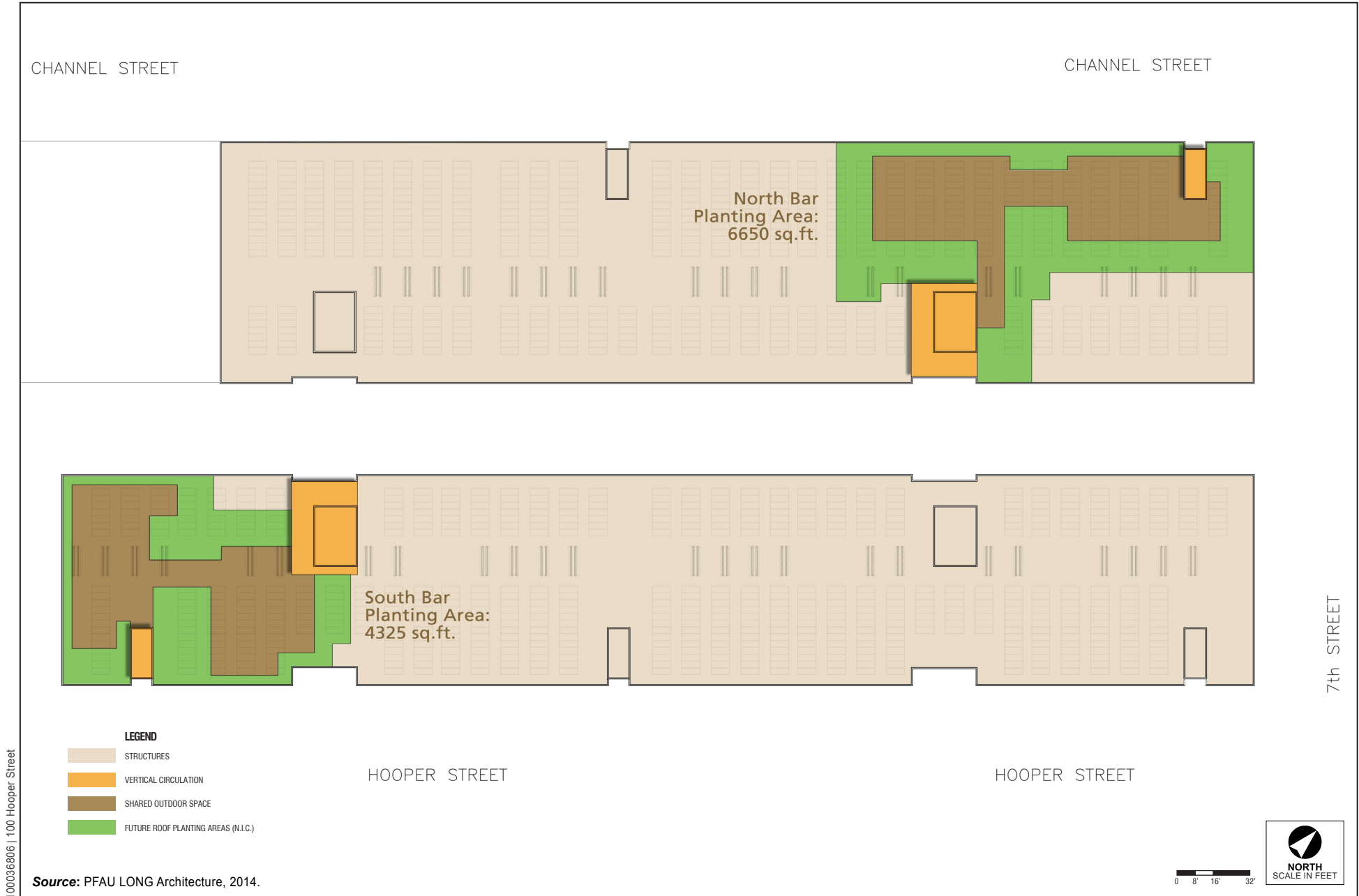
Figure 8c Preliminary Roof Deck Planting Area
